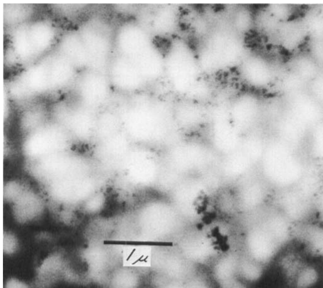
Fig. 7. Electron micrograph of a 1 : 1 mixture of Epon 815 and EM207 cured with TETA resin/curing agent ratio of 6 : 1 for 24 hr at 25^{\circ}\text{C} and 24 hr at 60^{\circ}\text{C} .
